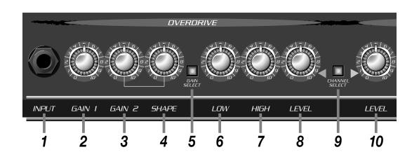
**1: INPUT:** Connect your guitar here by means of a shielded instrument cable.
